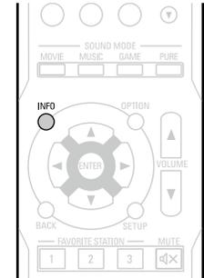
Status display: The operating status appears briefly on the screen when the input source is switched or the volume is changed.
