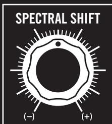
You can turn **SPECTRAL SHIFT** down from 12 o'clock just a little bit to simulate a formant shift to a deeper voiced person, or increase it a little bit above 12 o'clock to simulate an upwards formant shift to a higher voiced person.
