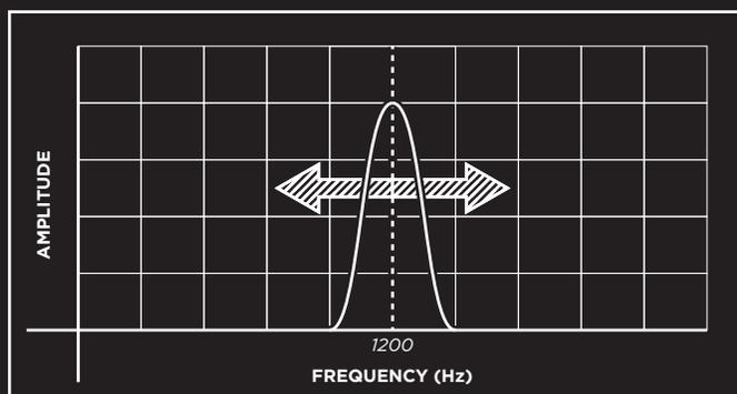
Spectravox is a unique exploration of the topology of the vocoder due to its filter design. Whereas most previous analog filter banks have their filters fixed in place, all 10 filters of Spectravox can be shifted up and down the frequency spectrum! Additionally, its filters all have variable **RESONANCE**, which provides for colorful sound design possibilities.
