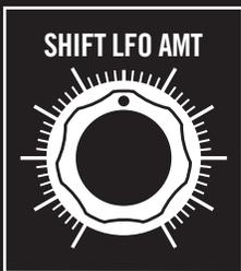
Here you have something like a comb filter—a handful of filters evenly spaced apart, with their peaks looking somewhat like a comb. Now, begin to move the **SHIFT LFO AMT** knob up—just a little bit at first, until you hear these five filters start to bend up and down together. Keep moving the **SHIFT LFO AMT** knob up to increase the range that the **LFO** shifts the filters.
