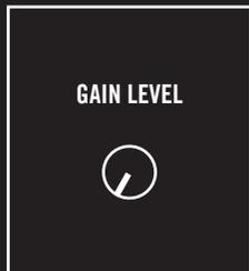
With the settings on page 18 and Spectravox's output connected to a monitoring system (or headphones), you should hear a vocoded signal as you speak into your microphone! If you don't, make sure to adjust the **GAIN LEVEL** control below the **PROGRAM INPUT** so that the LED indicates a nice strong signal—bright red at the loudest parts of your voice.
