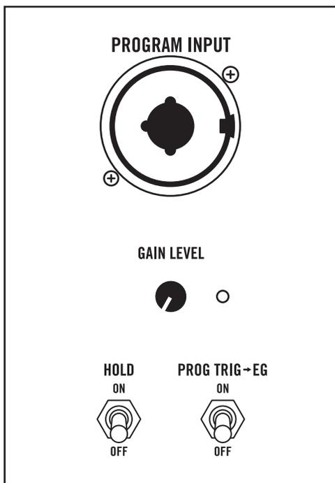
The **PROGRAM** section of Spectravox sends the signal connected to the **PROGRAM INPUT** into the analysis filter bank—whose outputs are the 10 envelope followers (**1 ENV F, 2 ENV F ... 10 ENV F**). The **PROGRAM** signal thus animates the synthesis filter bank when Spectravox is in **VOCODER** mode.
