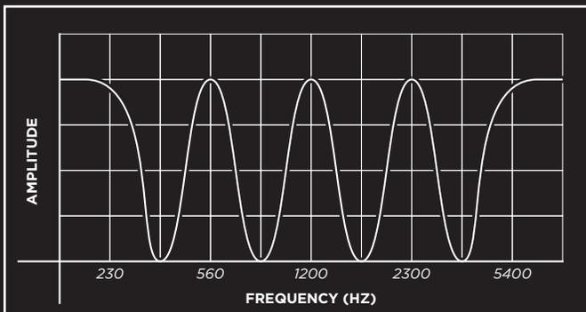
Play again with **RESONANCE** and **SPECTRAL SHIFT**. You will notice that all five filters move as you turn **SPECTRAL SHIFT**! This is the unique power of Spectravox: its filters are not fixed, but moveable.
