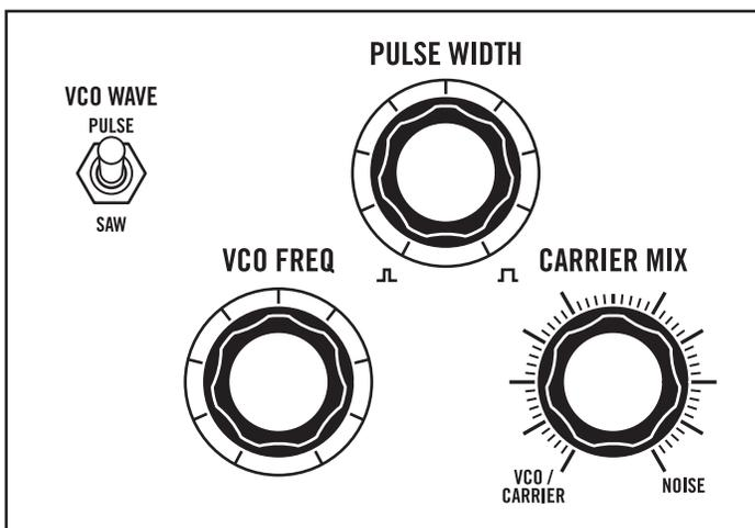
The **CARRIER** section of Spectravox generates a **CARRIER** signal which is sent to the synthesis filter bank and then sent to the **VCA** section and output. It consists of a variable waveshape **VCO**, a **NOISE** source, and **CARRIER MIX**.
