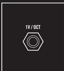
While modulating a static **CARRIER** signal with Spectravox is a lot of fun, you can start playing around with the **CARRIER** for more diverse tones. Adjust the **VCO FREQ**, or better yet, play it with a keyboard/sequencer by connecting a keyboard CV output (such as on Grandmother or Matriarch) or sequencer (using Mother-32, DFAM, or Subharmonic) to the **1V/OCT** input.
