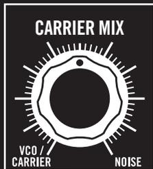
Move **SHIFT LFO RATE** up to increase the **LFO** rate, and move it down to decrease. Set the **SHIFT LFO RATE** down around eight o'clock and increase the **SHIFT LFO AMT** to around two o'clock to hear wide comb filter animation akin to a phaser effect. Shift the **CARRIER MIX** knob all the way counterclockwise to **VCO/CARRIER** to hear just the VCO, and as you move **RESONANCE** up you will hear a kaleidoscopic resonant sweep.
