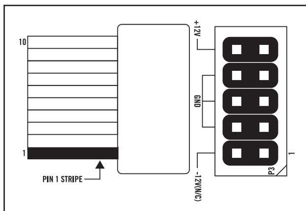
5. Look at the back of your Spectravox. There is a 10-pin power header on the back of the PCB that accepts a 10-pin Eurorack power ribbon cable (not included).
