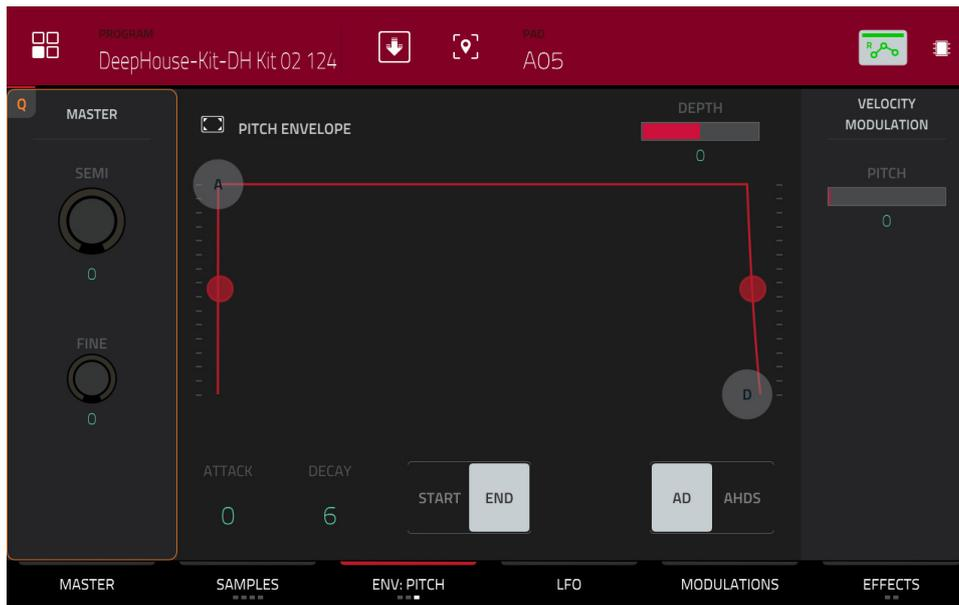
**Master Semi** lets you transpose the pad up to 36 semitones up or down. This will affect the length of the sample (if **Warp** is off). This is the same as the **Semi** field on the **Master** tab.
