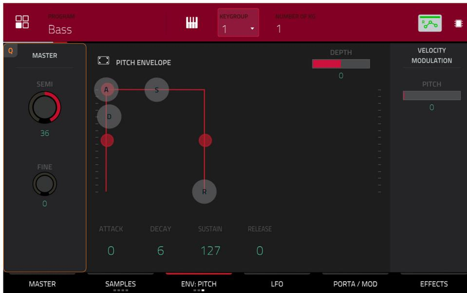
**Master Semi** lets you transpose the keygroup up to 36 semitones up or down. This will affect the length of the sample (if **Warp** is off). This is the same as the **Semi** field on the **Master** tab.
