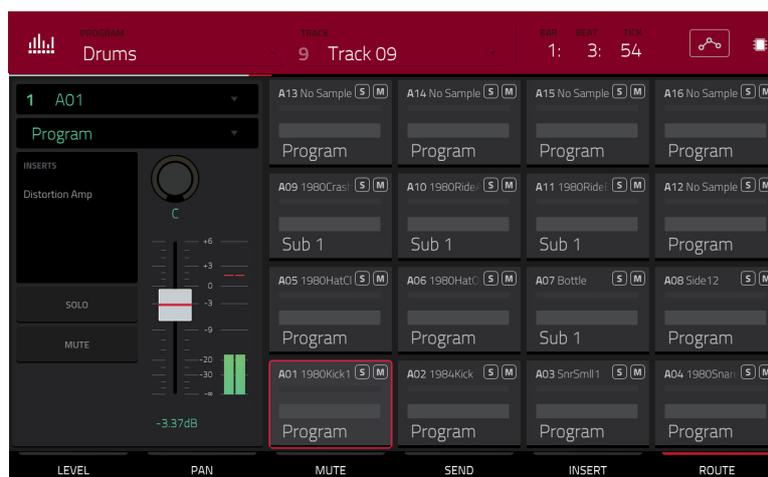
When the **Route** tab is selected, use the **data dial** or **-/+** buttons to select the output of the currently selected pad. Usually, this is set to **Program**. Double-tap a **pad** on the screen to select a different destination: **Out 1,2–7,8**, **Out 1–8** or **Sub 1–8** in Standalone Mode; and **Out 1,2–31,32** or **Out 1–32** in Controller Mode.
