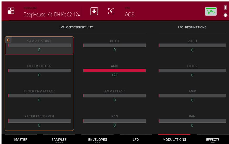
Use the **Velocity Sensitivity** sliders to set how much velocity is required to modulate certain other parameters:
