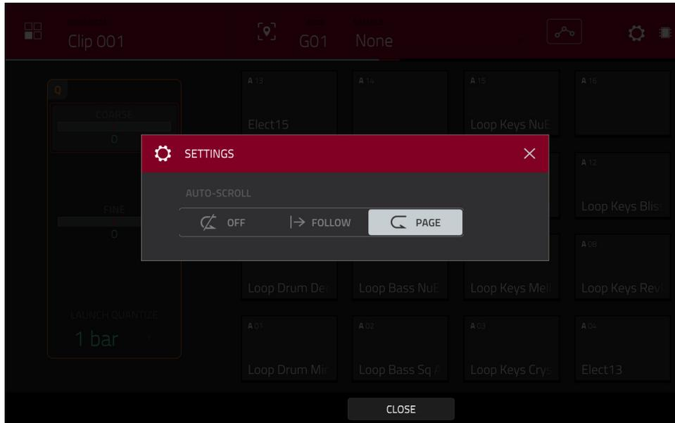
Use the **Auto-Scroll** selector to set how the screen behaves relative to the audio playhead while viewing the **Pad** tab.
