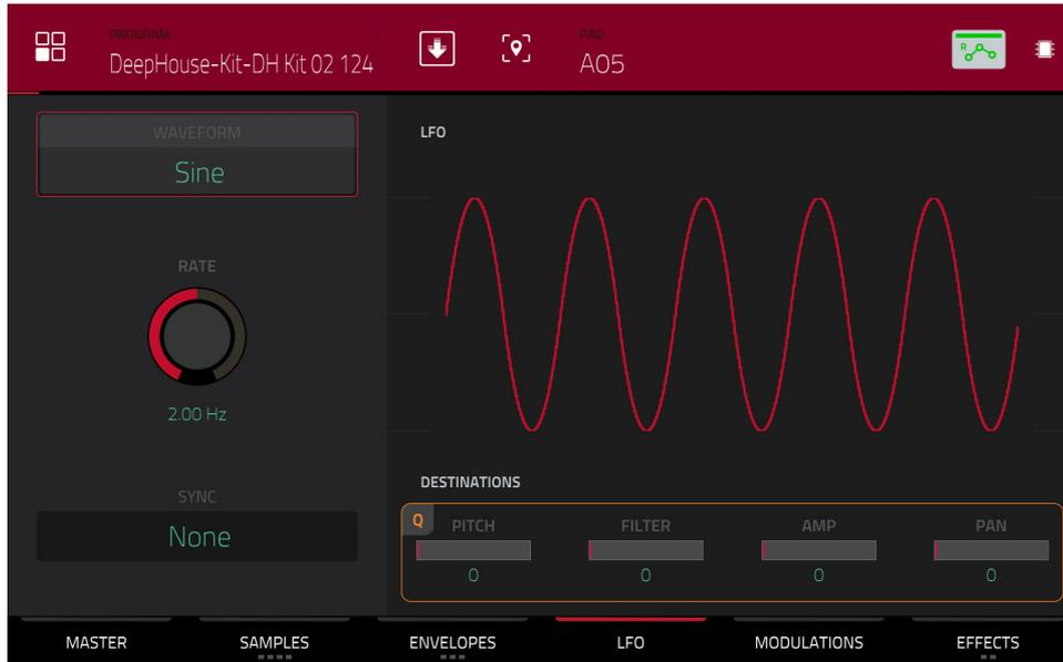
A low-frequency oscillator (LFO) generates a periodic waveform with an adjustable frequency and shape which can be used for modulation purposes.
