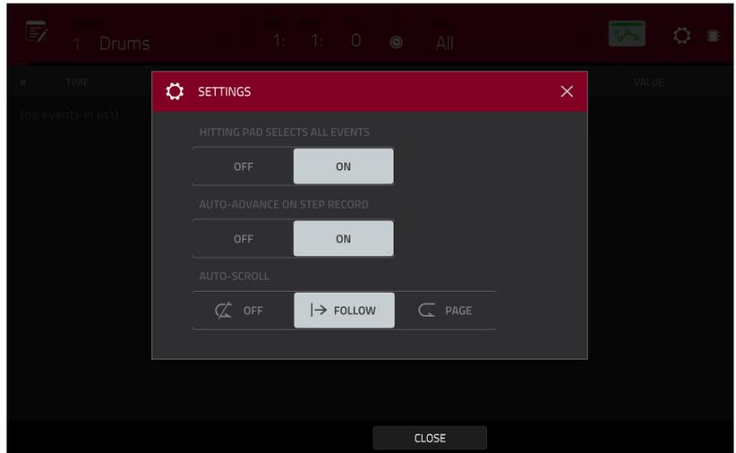
Use the **Hitting Pad Selects All Events** selector to turn the feature on or off. When **On**, pressing a pad will automatically select all note events for that pad in the sequence on that track. When set to **Off**, pressing a pad will simply play its sound without selecting any note events.
