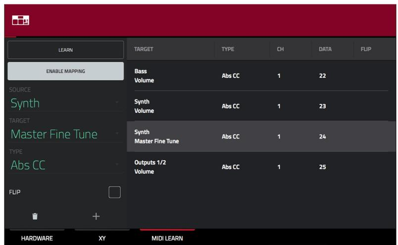
**Ch:** This is the MIDI channel the control is using.
