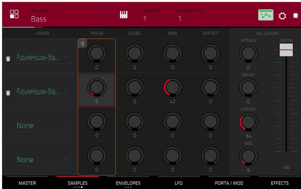
Use the **Pitch** knobs to adjust the amount of randomization applied to each sample layer's pitch.
