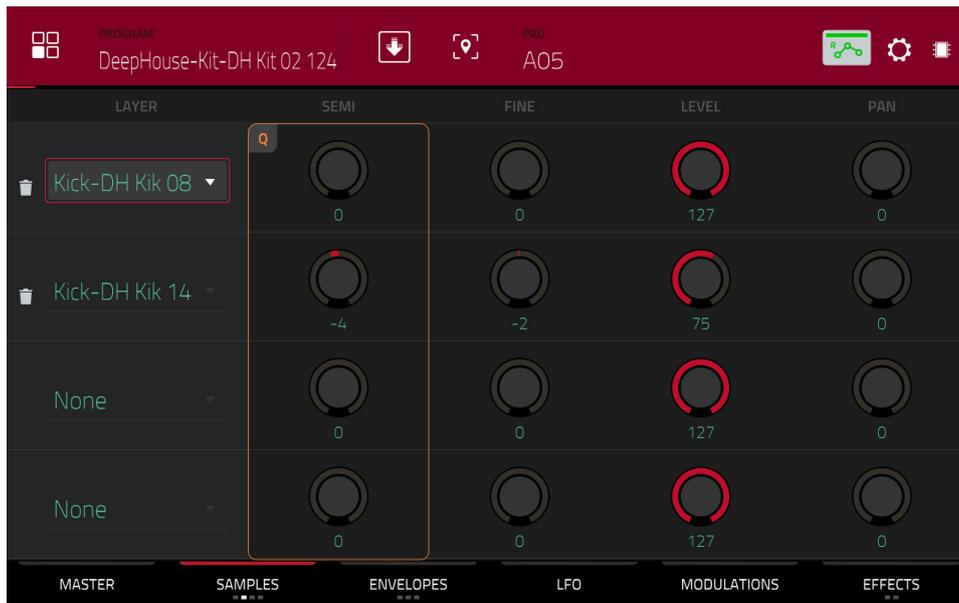
**Semi** lets you transpose the selected layer up to 36 semitones up or down. This will affect the length of the sample (if **Warp** is off). This is the same as the **Semi** field on the first Samples tab.
