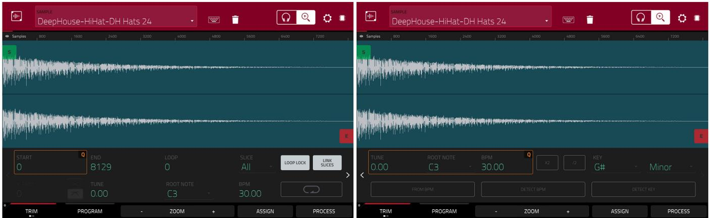
Use the **Start** and **End** fields to set the position of the start point and end point of the sample (respectively). Alternatively, tap and drag the start (**S**) or end (**E**) marker left or right, or use the **first** column of **Q-Link knobs (Start X1\_\_)** to adjust the start point or the **second** column of **Q-Link knobs (End X1\_\_)** to adjust the end point.
