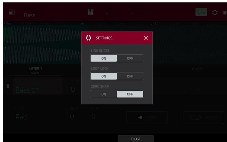
Use the **Link Slices** selector to set how the start point and end point of a slice in a larger sample is set. You can create these slices in Sample Edit Mode (Chop Mode).
