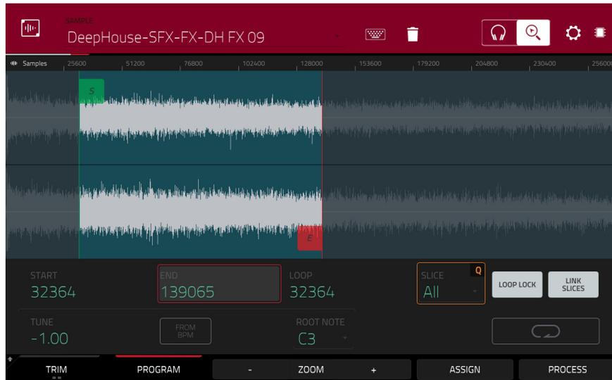
Use the **Start** and **End** fields to set the position of the start point and end point of the sample (respectively). Alternatively, tap and drag the start (**S**) or end (**E**) marker left or right, or use the **first** column of **Q-Link knobs** (**Start X1\_\_**) to adjust the start point or the **second** column of **Q-Link knobs** (**End X1\_\_**) to adjust the end point.
