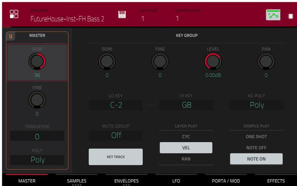
**Semi** lets you transpose the sample 36 semitones up or down, while **Fine** provides fine-tuning of each layer up to 99 cents up or down.
