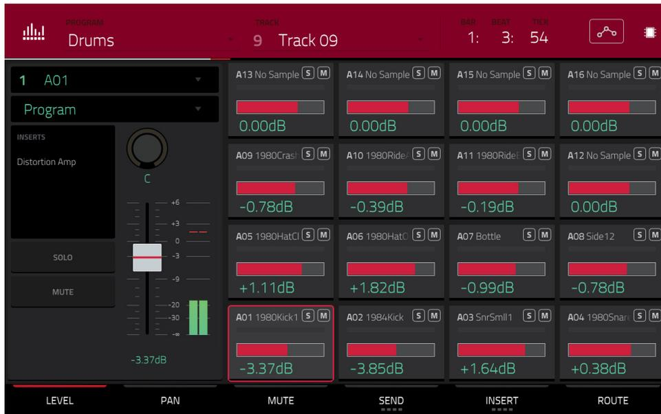
When the **Level** tab is selected, use the **data dial** or **-/+** buttons to adjust the level of the currently selected pad.
