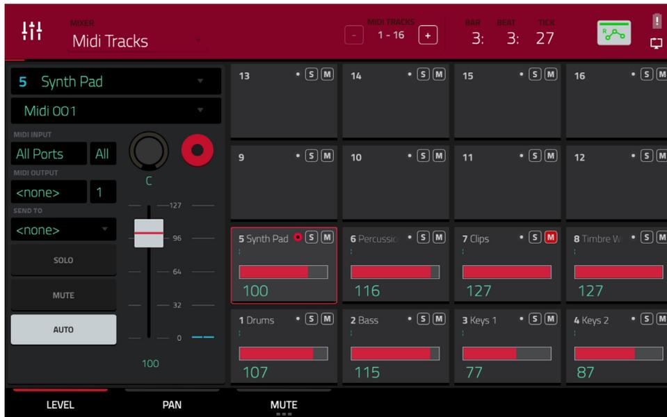
The Channel Mixer works like an audio mixer with various settings for each channel, shown in a 4x4 array. Their functionality is mostly identical. The name of the track, program, or channel is displayed at the top of each one.
