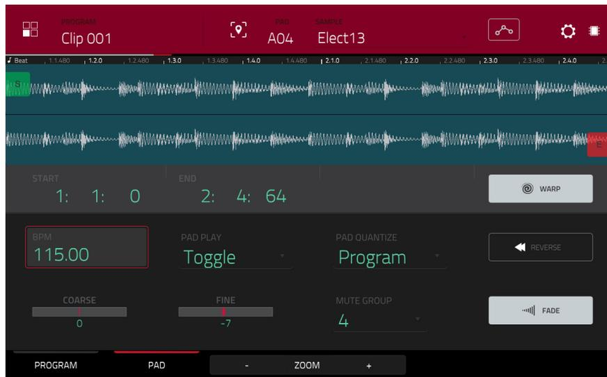
Tap **Warp** to lengthen or shorten the clip without changing its pitch, and use the **BPM** field to change the tempo. Use the **Coarse** and **Fine** sliders if you want to change the pitch.
