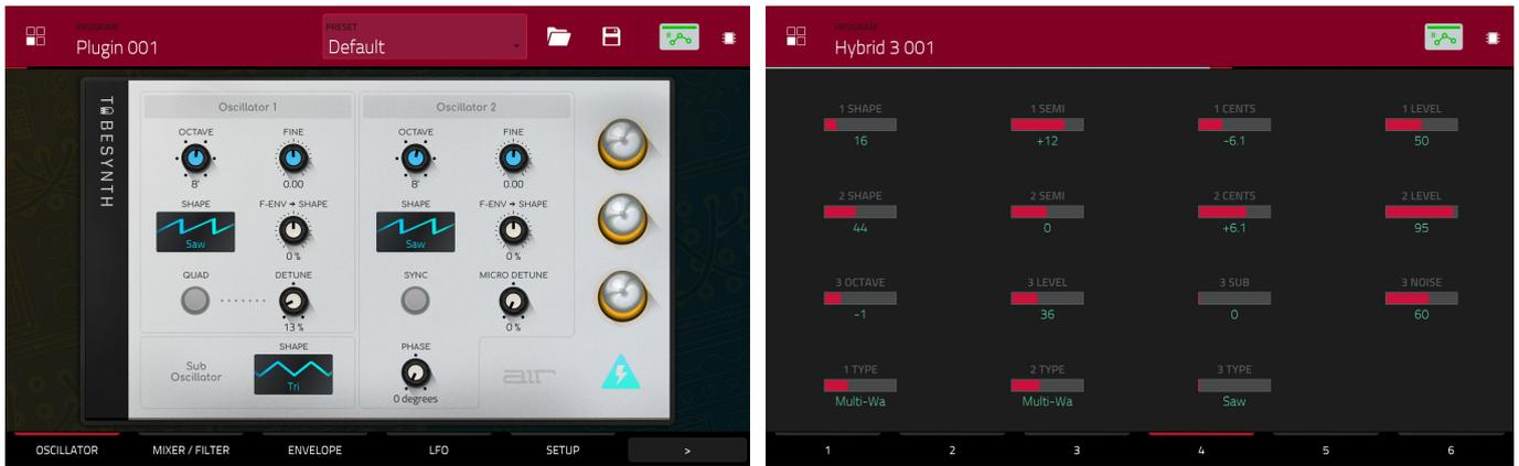
For plugin programs, you will see a graphical representation of the plugin interface, or an overview of all available plugin parameters with a slider for each.
