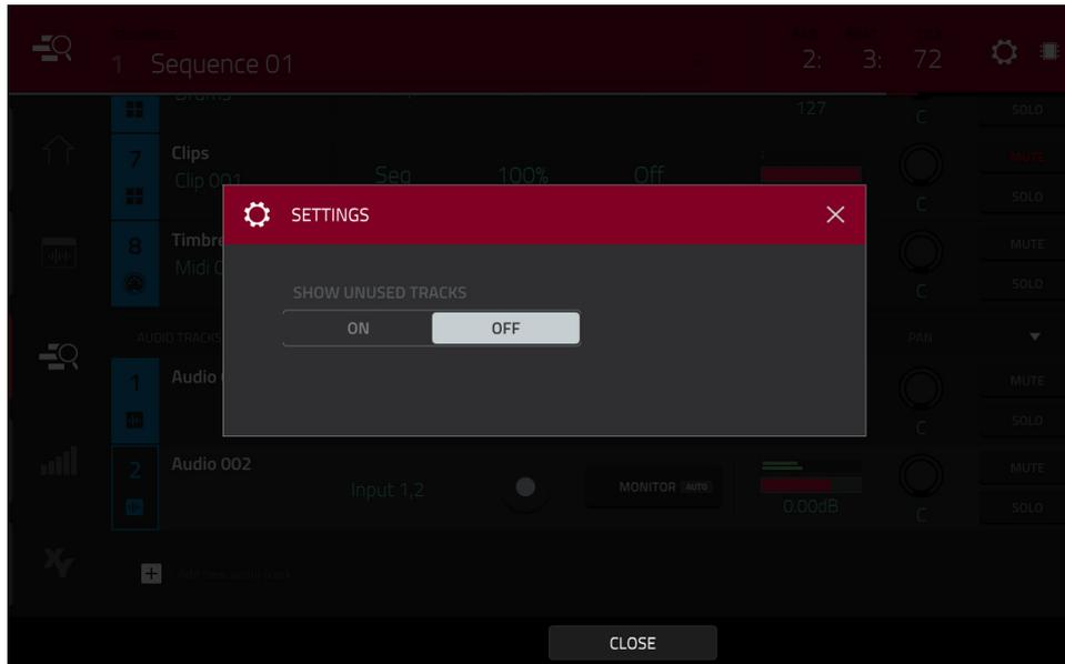
Use the **Show Unused Tracks** selector to turn this feature on or off. When **on**, tracks with a sequence, program, etc. will still appear in the Track View. When **off**, only tracks with a sequence, program, etc. will appear.
