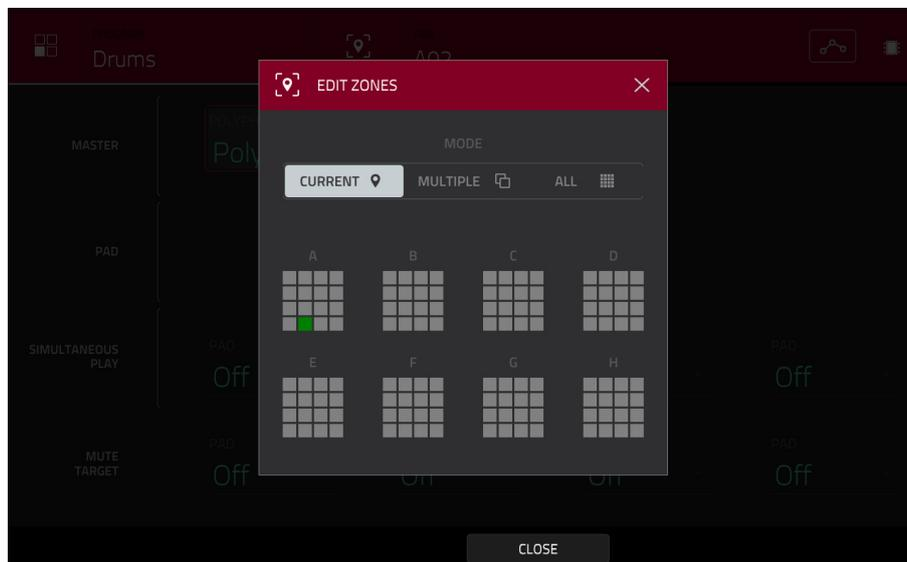
Tap the **location icon** at the top of the screen (between the **Program** and **Pad** fields) to open the **Edit Zones** window, which is a feature for drum programs and clip programs. This window displays an overview of any selected pads. Use the **Mode** selector to set how the selected pads will be edited:
