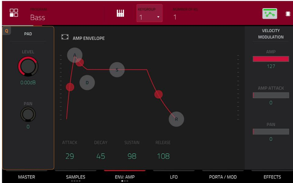
The **first Envelope** tab contains the amplitude modulation envelope.
