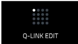
Q-Link Edit Mode lets you determine what the Q-Link knobs control in other modes. This is helpful when you want to use the Q-Link knobs to control parameters that might not be shown in the current mode—or parameters that are shown across different modes.
