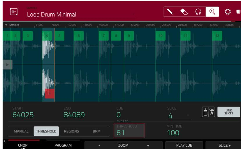
Use the **Start** and **End** fields to set the position of the start point and end point (respectively) of the currently selected slice. Alternatively, tap and drag the start (**S**) or end (**E**) marker left or right, or use the **first** column of **Q-Link knobs (Start X1\_\_)** to adjust the start point or the **second** column of **Q-Link knobs (End X1\_\_)** to adjust the end point.
