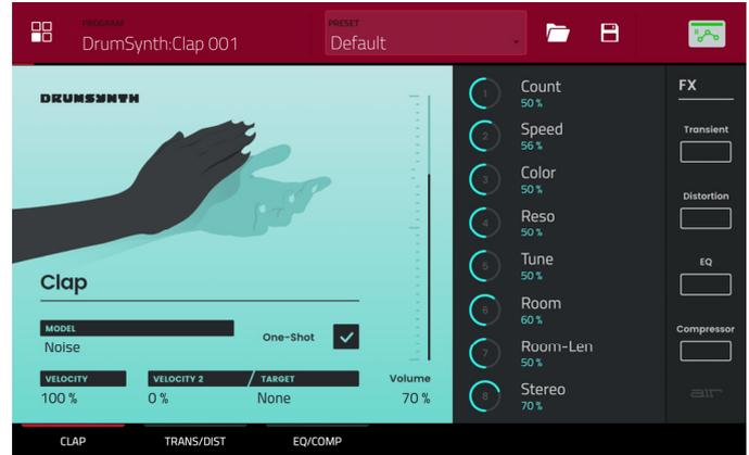
In each plugin, you can quickly enable or disable the built-in effects (**Transient**, **Distortion**, **EQ** and **Compressor**) while viewing any of the tabs listed below by tapping the buttons on the right side of the touchscreen under **FX**.
