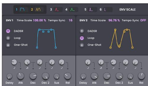
Use these tabs to adjust the six amplitude modulation envelopes. Tap the tab to cycle between each, or tap the envelope icons at the top of the window.
