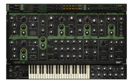
Like many classic hardware synths, Vacuum Pro has a straightforward layout in which you can see the flow of your signal from left to right and there is only one "mode" of operation (i.e., no separate "play" or "edit" modes). Furthermore, nearly all of the buttons and knobs have only one function. These design elements make it easy to develop "muscle memory" and confidently reach for the right knob without having to actively think about what you're doing.
