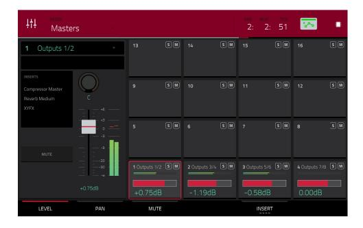
The Master Mixer shows levels, panning, mute states, and insert effects for all used stereo pairs of outputs (**Out 1,2–7,8** in Standalone Mode, **Out 1,2–31,32** in Controller Mode; MPC Live does not use Out 7,8 and MPC One does not use Out 3,4–7,8 in Standalone Mode, but displays them to maintain compatibility with MPC X, which does use them).
