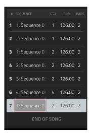
Each used sequence is assigned to a pad. Empty pads correspond to unused sequences. Use the **Pad Bank** buttons to access the sequences assigned to pads in other banks.
