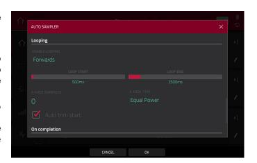
Use the **Loop start** and **Loop end** sliders to set the starting and ending points in the sample where the loop will occur.
