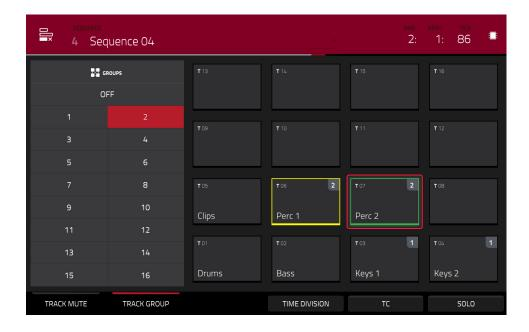
The track group feature extends the concept of track mutes: you can mute or unmute multiple tracks (in a single sequence) by pressing one pad that you have assigned to a track group. This is useful if you want to hear a track without a particular group of sounds or if you want to isolate specific sounds in various combinations. You can create up to 16 different track groups.
