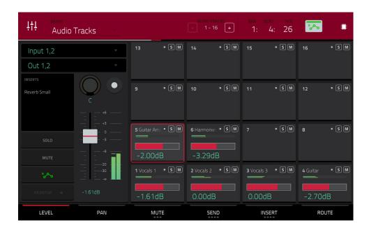
The Audio Track Mixer shows levels, mute/solo/record-arm states, send and insert effects, and routing for all used tracks.
