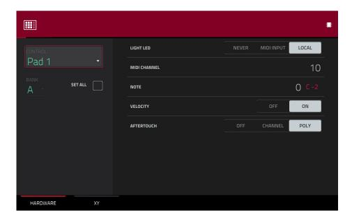
In the touchscreen, use the fields and selectors to set each control's parameters to your preference. The available parameters depend on its type: a **pad**, or **button**, a **Q-Link knob**, or each axis of the **XY pad**. When you have set all of the parameters as desired, you can select another control or enter another mode.
