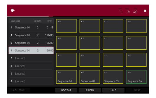
The time counter in the upper-right corner the current playhead position. This is shown in most of the modes. See *General Features > Time Counter/Locate* to learn about this.
