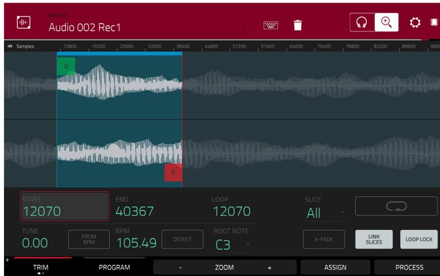
Use the **Root Note** field to set the root note of the sample. This defines which note will play the sample at its original pitch when in a keygroup program.
