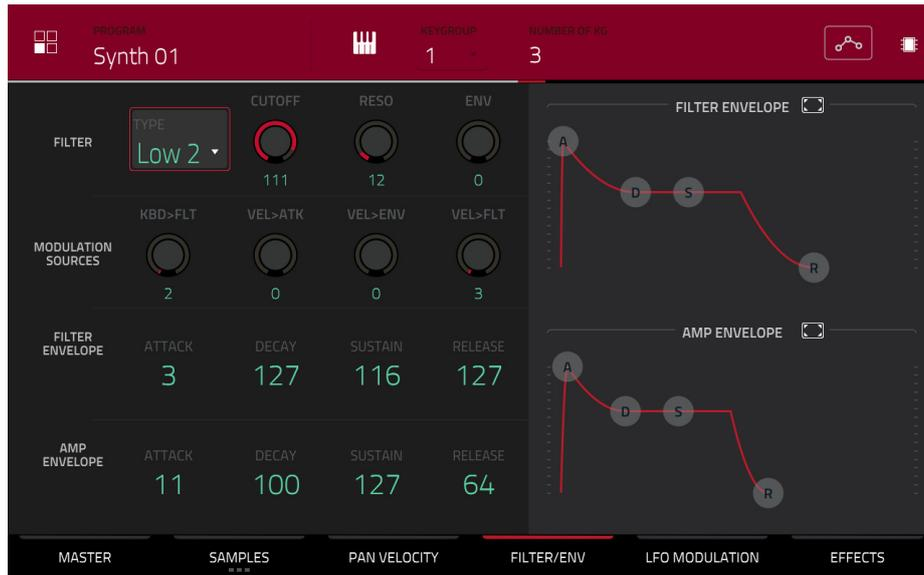
Use the **Type** field to select a filter for the selected pad. See [Appendix > Glossary > Filter](#) for an explanation of the available filter types.
