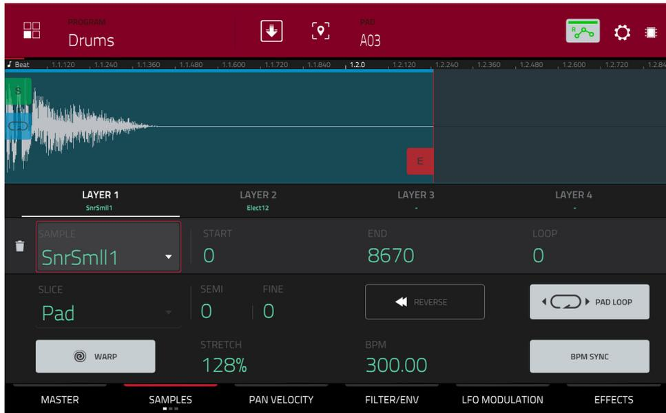
Use the **Reverse** button to select in which direction the sample will play. When on, the sample will play in reverse. When off, the sample will play in the normal forward direction.
