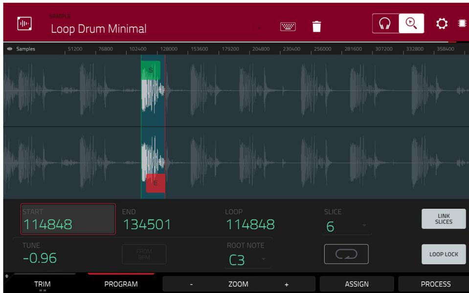
The **Link Slices** button does not have a function in Program Mode.
