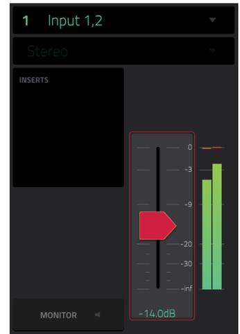
The **Inserts** field shows any enabled or disabled effects for the Sampler. Tap the area under **Inserts** to open a window where you can load, change, and enable or disable the effects.
