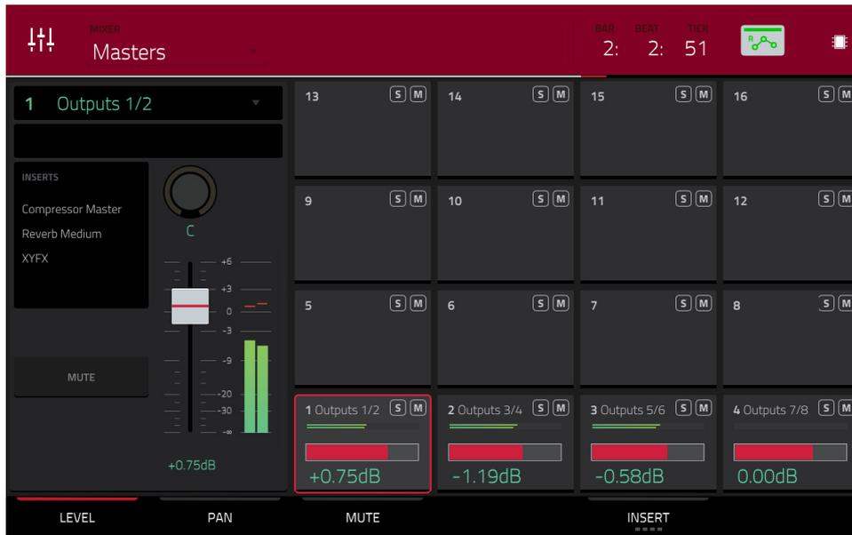
The Master Mixer shows levels, panning, mute states, and insert effects for all used stereo pairs of outputs (**Out 1,2–7,8** in Standalone Mode, **Out 1,2–31,32** in Controller Mode; MPC Live does not use Out 7,8 in Standalone Mode but displays them to maintain compatibility with MPC X, which does use them).
