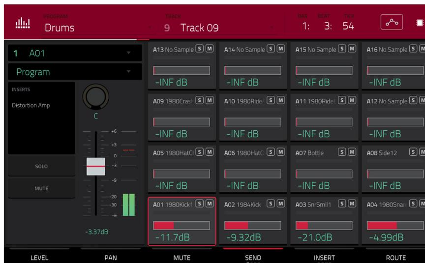
When the **Send** tab is selected, use the **data dial** or **-/+** buttons to adjust the send level of the currently selected pad. The level sliders in each pad show a visual representation of the level. Double-tap a **pad** on the screen to open a large version of the level slider.
