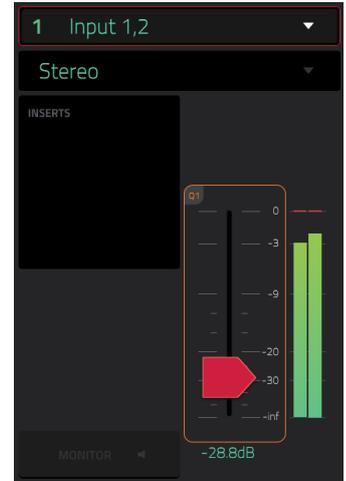
The **Inserts** field shows any enabled or disabled effects for the Looper. Tap the area under **Inserts** to open a window where you can load, change, and enable or disable the effects.
