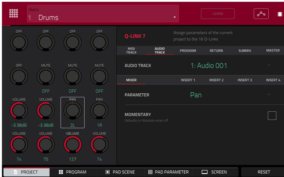
Next to the top row of Q-Link knobs on the screen, tap one of these tabs to select the type of parameters you want to control with the Q-Link knobs:
