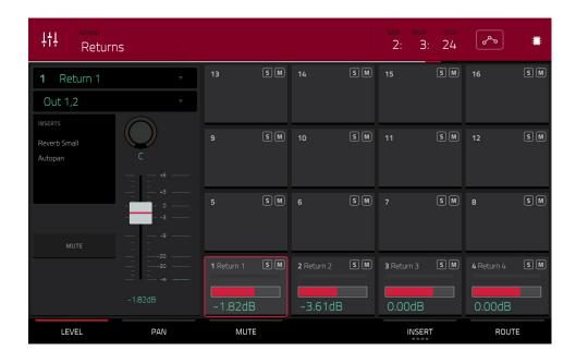
Pads, programs, and audio tracks can each be sent to up to four send channels. Their audio signals will be routed to the send channels at their designated send levels. After being processed by the effects on those channels, their signals are then sent to the assigned master output based on their return settings (levels, panning, etc.). This view displays the four return channels. The return mixer shows levels, panning, mute states, insert effects, and routing for all used tracks.
