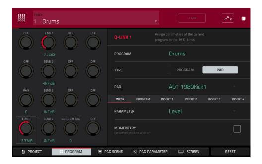
To select an edit mode for the Q-Link knobs, tap one of the five buttons at the bottom of the screen. If you are using MPC X, you can also press one of the five Q-Link buttons above the Q-Link knobs (Project, Program, Pad Scene, Pad Param, or Screen Control/Edit):
