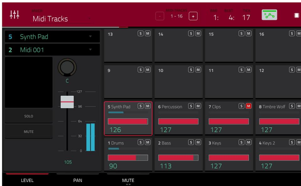
The Channel Mixer works like an audio mixer with various settings for each channel, shown in a 4x4 array. Their functionality is mostly identical. The name of the track, program, or channel is displayed at the top of each one.
