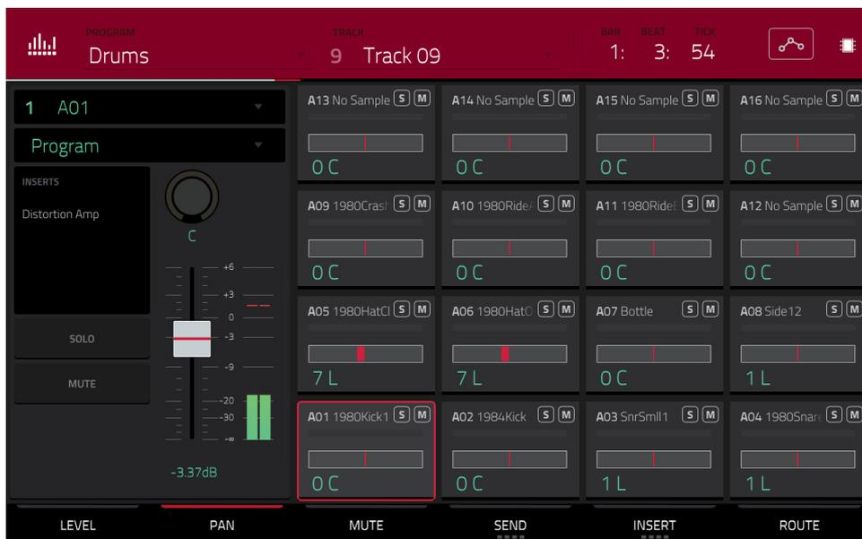
When the **Pan** tab is selected, use the **data dial** or **-/+** buttons to adjust the panning of the currently selected pad.
