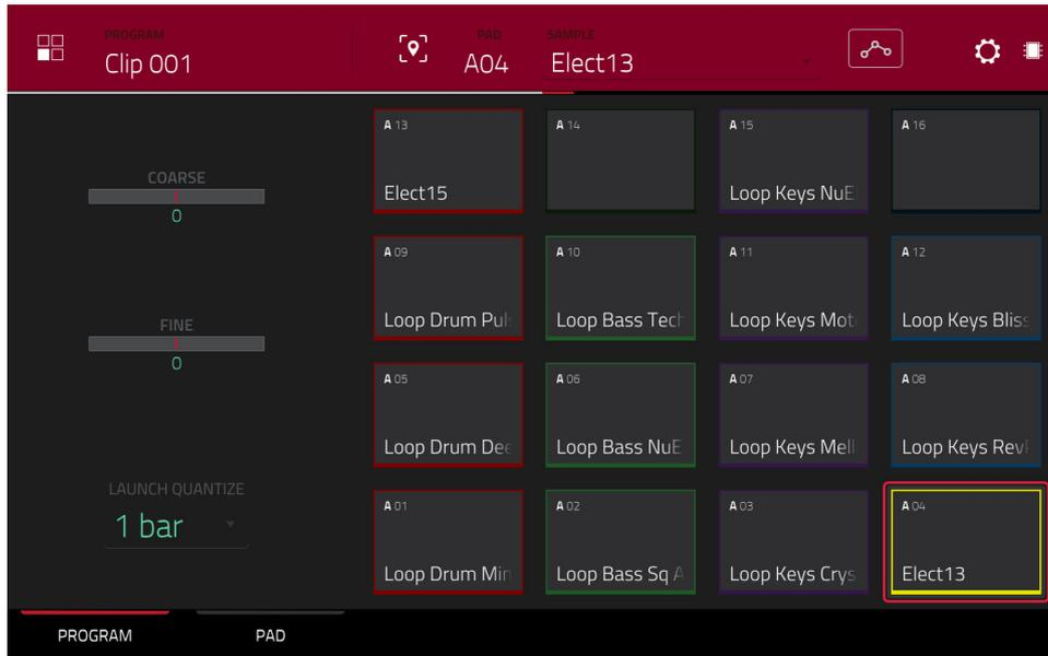
**To assign a sample to a pad**, press or tap a pad to select it (it will play its assigned samples, if any). Tap the **Sample** field, and then use the **data dial** or **-/+** buttons to select a clip. Alternatively, double-tap the **Sample** field, and then tap a clip to select it.
