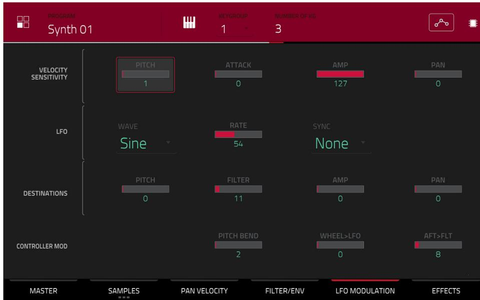
Use the **Rate** field to determine the LFO frequency. At lower values, it might take some time for the LFO to complete a cycle, while higher values will come closer to audible range.
