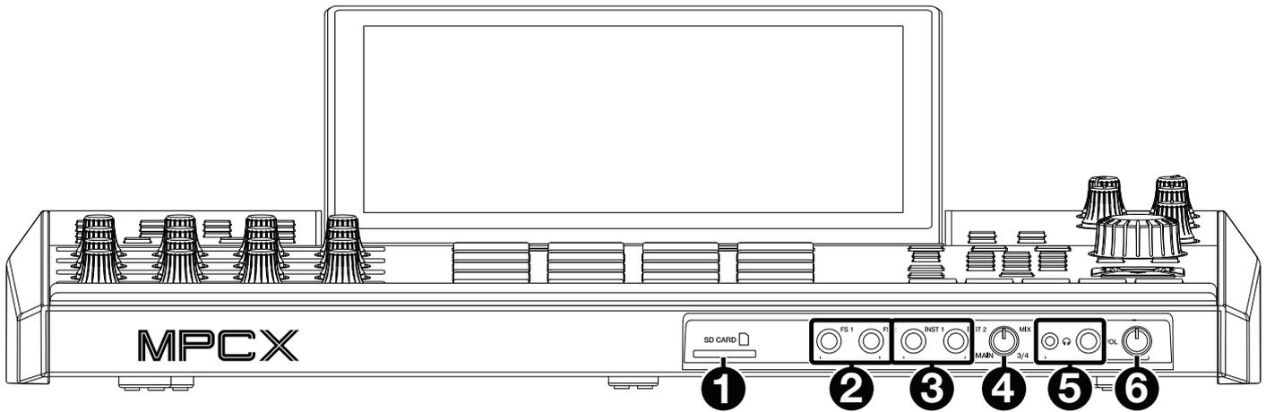
1. **SD Card Slot:** Insert a standard SD/SDHC card into this slot to access its files directly using MPC X.
