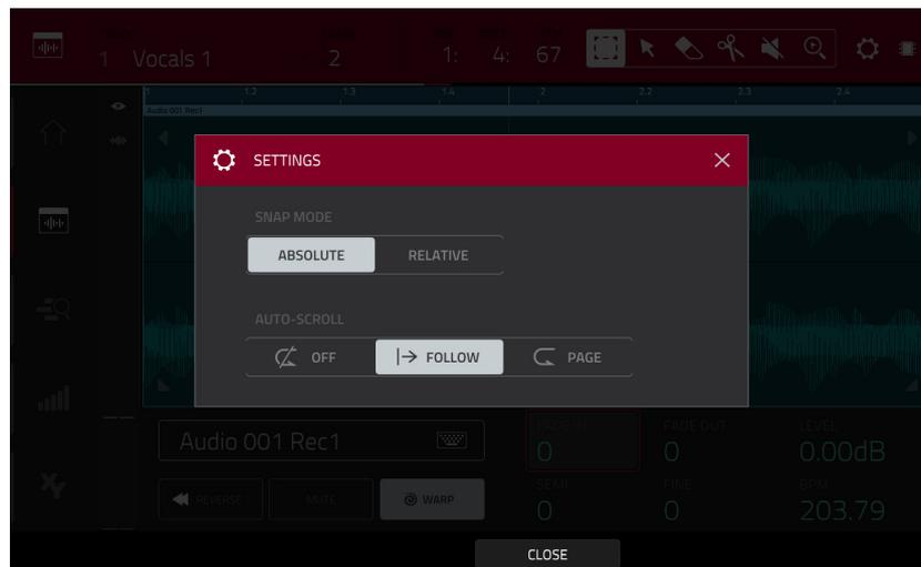
Use the **Snap Mode** selector to set how events “snap” to the grid.
