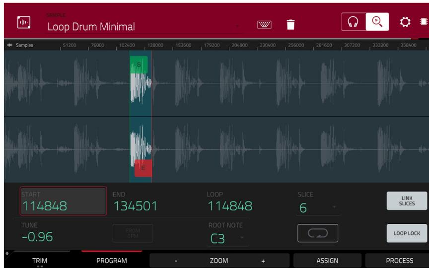
Use the **Start** and **End** fields to set the position of the start point and end point of the sample (respectively). Alternatively, tap and drag the start (**S**) or end (**E**) marker left or right, or use the **first** column of **Q-Link knobs (Start X1\_\_)** to adjust the start point or the **second** column of **Q-Link knobs (End X1\_\_)** to adjust the end point.
