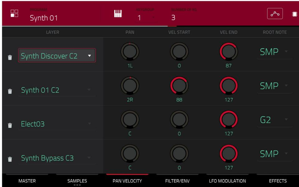
Use the **Pan knob** to adjust the stereo placement of the respective layer.
