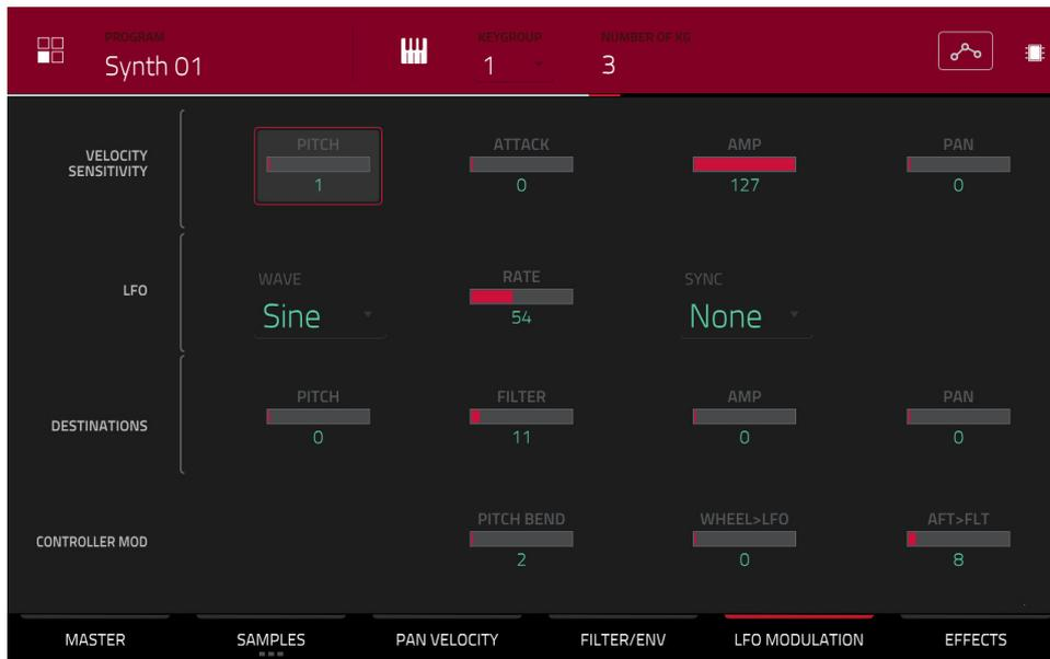
The **Velocity Sensitivity** controls determine how much the velocity affects the pitch of the sound (**Pitch**), the attack of the filter envelope (**Attack**), the volume level of the sound (**Amp**), and the panning of the sound (**Pan**).
