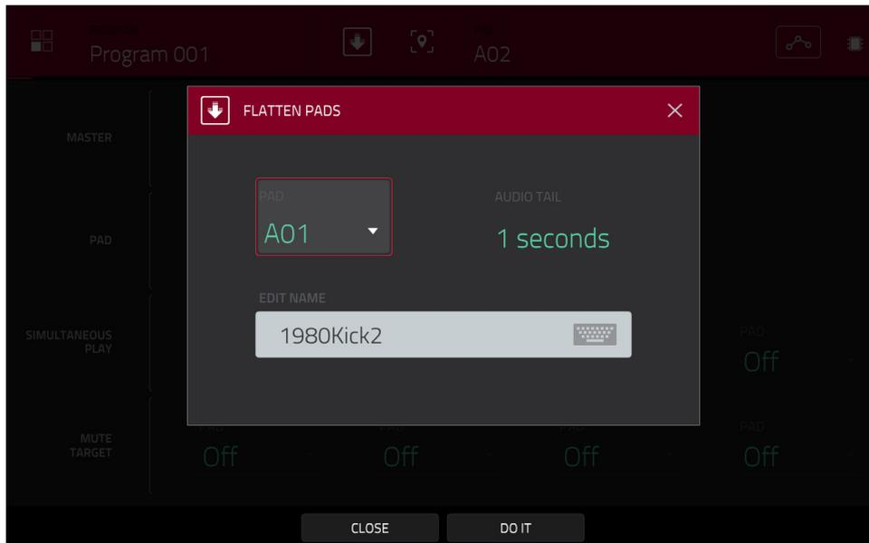
Tap the **down-arrow icon** at the top of the screen (next to the **Program** field) to open the **Flatten Pad** window, which renders all samples on a pad as an audio sample and places it on the first layer of that pad. The resulting sample is the audio signal produced by that pad at full velocity (**127**) after the pad channel strip, which means that it includes any assigned pad insert effects and the results of warping the sample.
