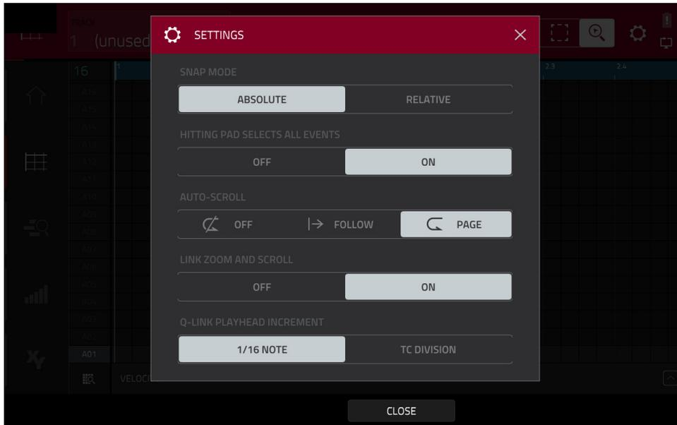
Use the **Snap Mode** selector to set how events “snap” to the grid.
