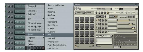
\*Each pad on the MPD32/MPK49 sends a MIDI Note #. You can view this number by pressing the pad and reading the displayed Note # on the LCD screen. Each virtual pad in the FPC responds to a MIDI Note #. You can view this number by clicking the virtual pad and reading the MIDI Note displayed in the upper right corner.
