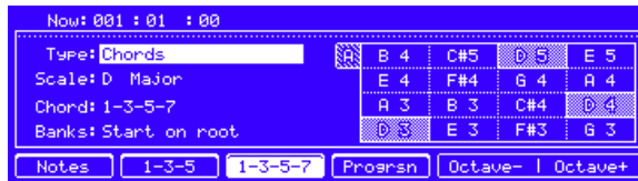
First bank of buttons in Pad Perform Mode in the MPC hardware display.
