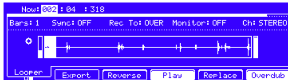
The Looper tab in Sample Record Mode in the MPC hardware display.
