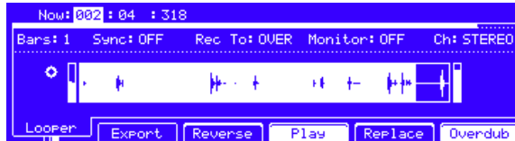
The Looper tab in Sample Record Mode in the MPC hardware display.
