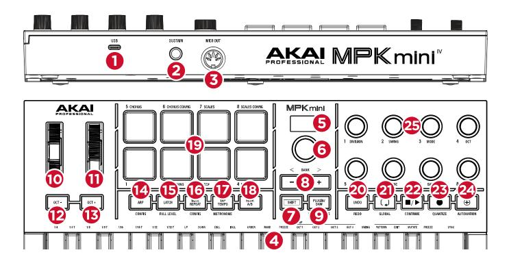
1. **USB-C® Port:** Use the included cable to connect this port to a USB port on your computer. This will allow you to send and receive MIDI data and communicate with software, such as the included Studio Instrument Collection or Ableton Live.
