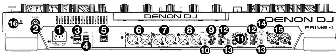
1. **Power Input:** Use the included power cable to connect this input to a power outlet.
