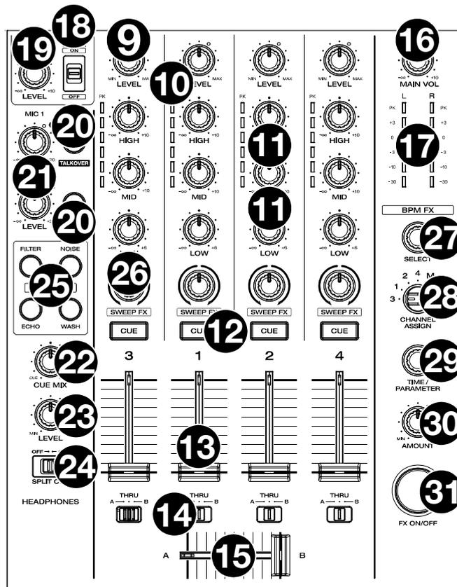
21. **Mic 1 / Aux/Mic 2 Level:** Turn this knob to adjust the volume level for the **Microphone 1–2** and **Aux** inputs. The **Peak** light next to each knob indicates the current signal level by its color: **green** (low), **amber** (normal/optimal), or **red** (maximum/peak). You can adjust additional microphone and aux settings in the **Settings** menu.
