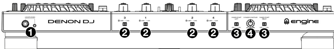
1. **Headphones (1/4", 1/8") (6.35 mm, 3.5 mm):** Connect your 1/4" or 1/8" (6.35 mm or 3.5 mm) headphones to this output for cueing and mix monitoring. The headphone volume is controlled using the **Phones Level** knob.
