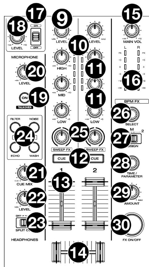
21. **Cue Mix:** Turn this knob to adjust the blend of the pre-fader and main mix together in the headphones.
