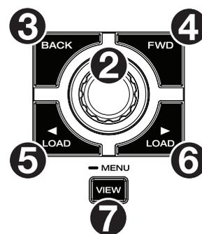
5. **Load ◀:** Press this button to load the selected track to Deck 1 or Deck 3.
