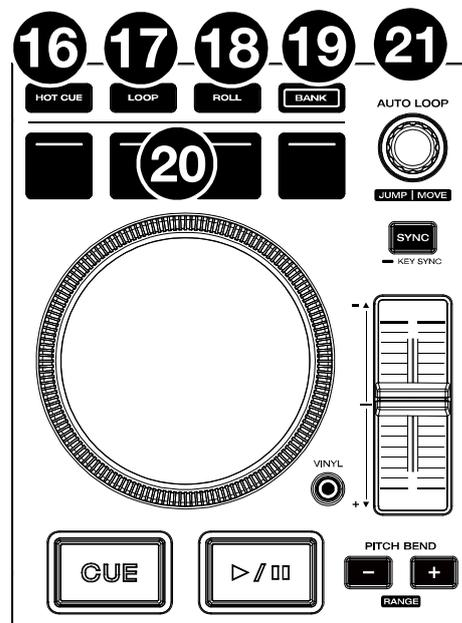
22. **Sync:** Press this button to activate sync. When Key Lock is activated, the track's key will remain the same even if you adjust its speed.
