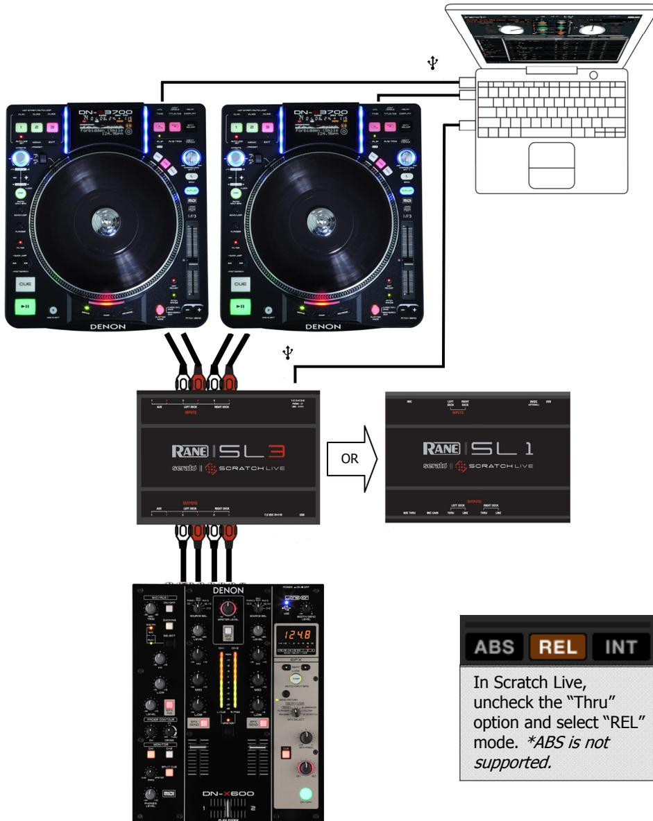
**DN-S1200:** Connect the analog RCA Outputs from the Left and Right Decks to the Rane/Serato SL3, SL1 (TTM57SL, TTM68) Inputs. Connect a USB cable from each Deck and Rane/Serato hardware to your computer.
