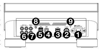
2. **Power Button**: Press this button to power SC6000 PRIME on or off. Power on SC6000 PRIME only **after** you have connected all of your input devices and **before** you power on your amplifiers and loudspeakers. Power off your amplifiers and loudspeakers **before** powering off SC6000 PRIME.
