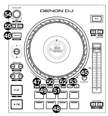
Press and hold Shift and then press this button to reverse the playback of the track normally.
