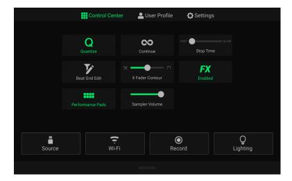
**Quantize:** Tap this to enable or disable quantization. When enabled, time-based features like triggering cues and loops will snap to the beat-grid according to the **Cue/Loop Quantization** setting in your **User Profile**.
