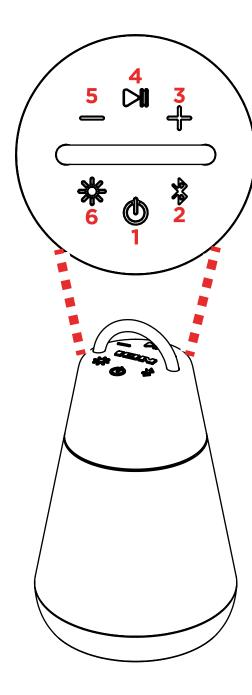
1. Power: Press this button to turn the Luma Duo speakers on. Press and hold this button to turn the Luma Duo speakers off.
