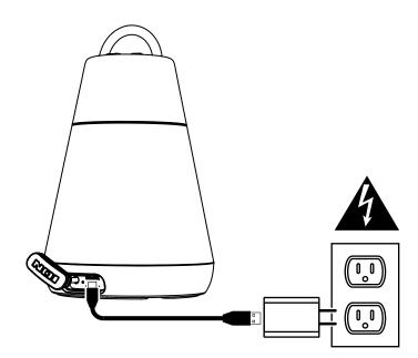
**Important:** For best results, power off the Luma Duo speakers and use the included USB-A to USB-C® charging cable to connect the **USB-C® Charging Port** on the rear panel of each speaker to a USB power adapter (DC 5V, 2A; not included) connected to a power outlet. A full charge can take up to 3 hours, depending on the specifications of your 5V, 2A adapter.
