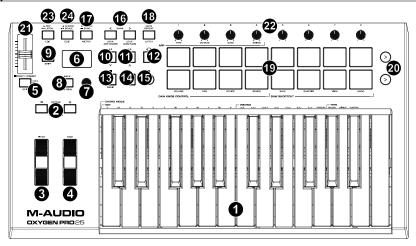
**Note:** Text below accompanying keyboard controls indicates secondary functions that can be accessed by pressing **SHIFT** while using the control.
