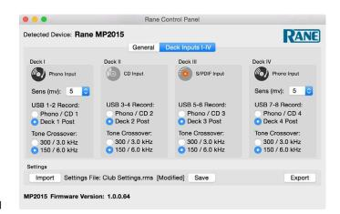
Sensitivity to the same level of your cartridge (see your cartridge documentation for the correct value). Another method is to match the level of the turntable to a CD playing on another input.
