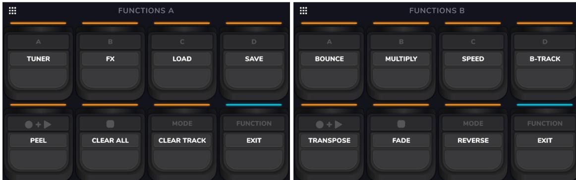
To select a function, press the corresponding **pedal** (labeled on the top panel in orange) or tap it on the touchscreen.
